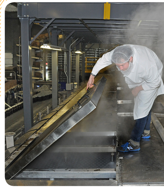
Yoshida quality assurance supervisor Sean Brown checks the spray patterns of the new pasteurizer.
